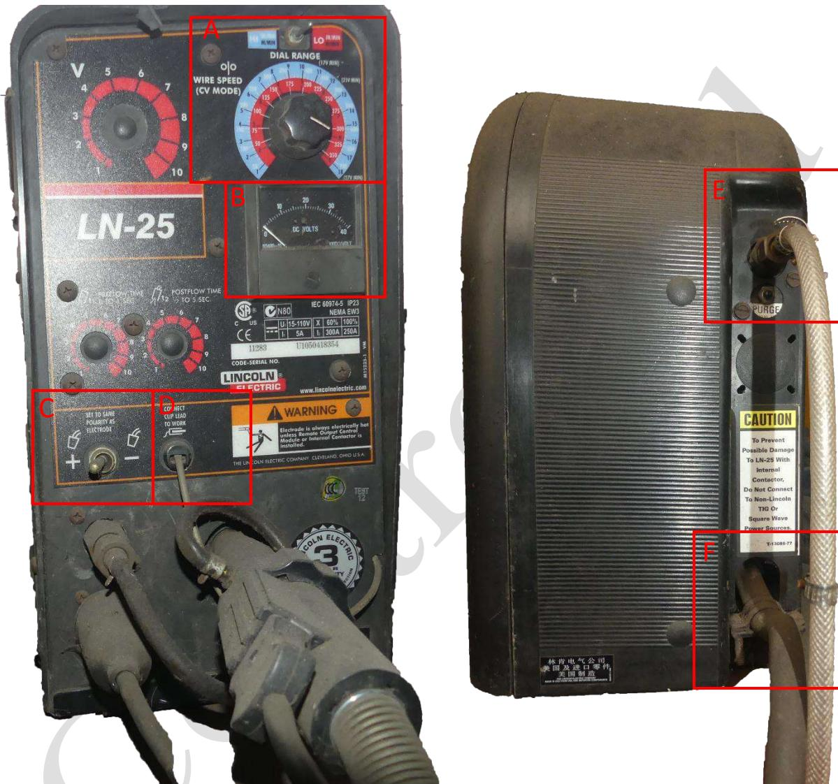
*Gambar 3. Penjelasan panel Wire Feeder Lincoln LN25*
