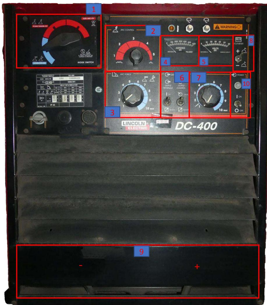
Gambar 2. Penjelasan panel Mesin Las Lincoln DC400
